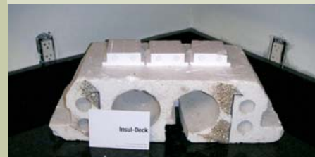
Sample of cement/polystyrene ceiling (with space for wiring and conduit).
