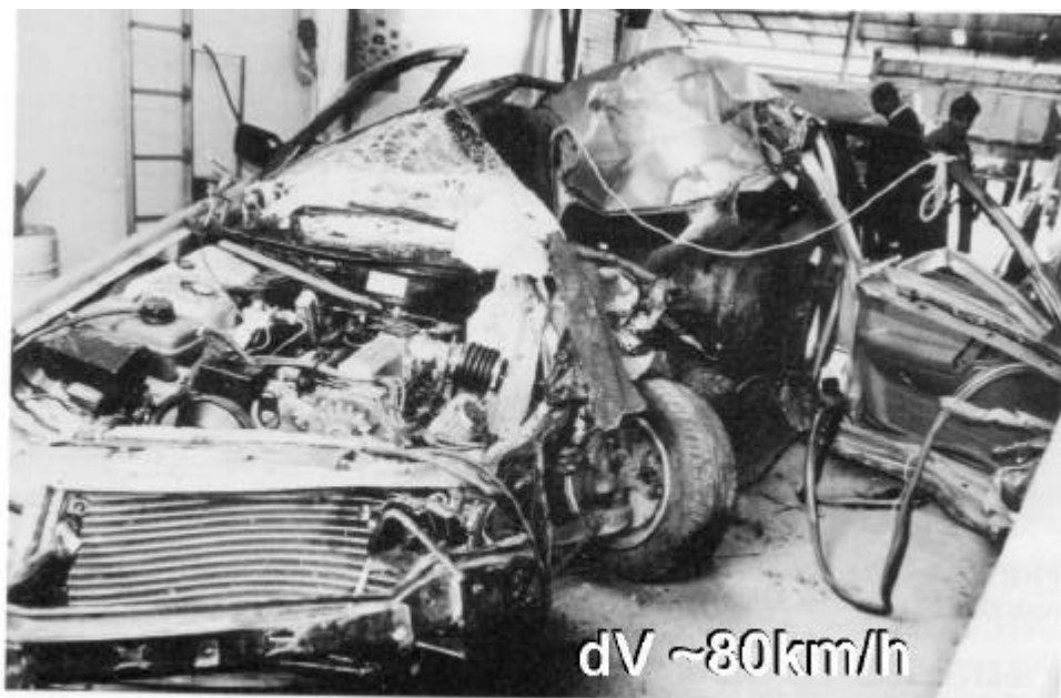
FIGURE 8 - Collision with tree in country; child in restraint in centre rear position uninjured (13513)
