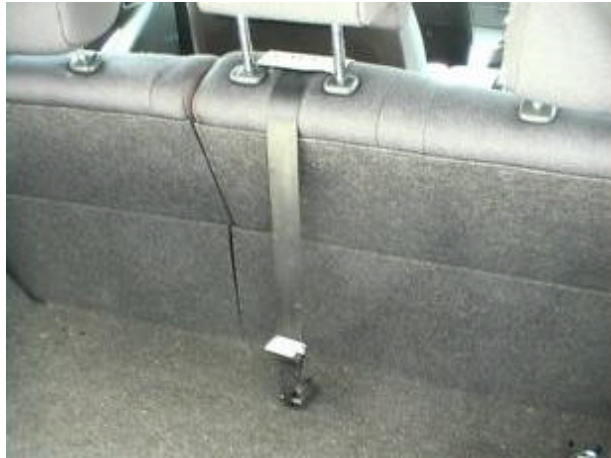
Top tether relies on seat structure to resist forward movement
