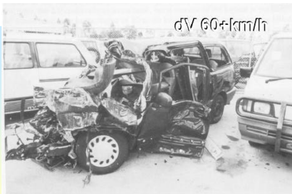
FIGURE 11 - Toyota Tarago in which three adults killed; three-year old centre seat, second row, sustained broken arm and lacerations from flying glass (28214)
