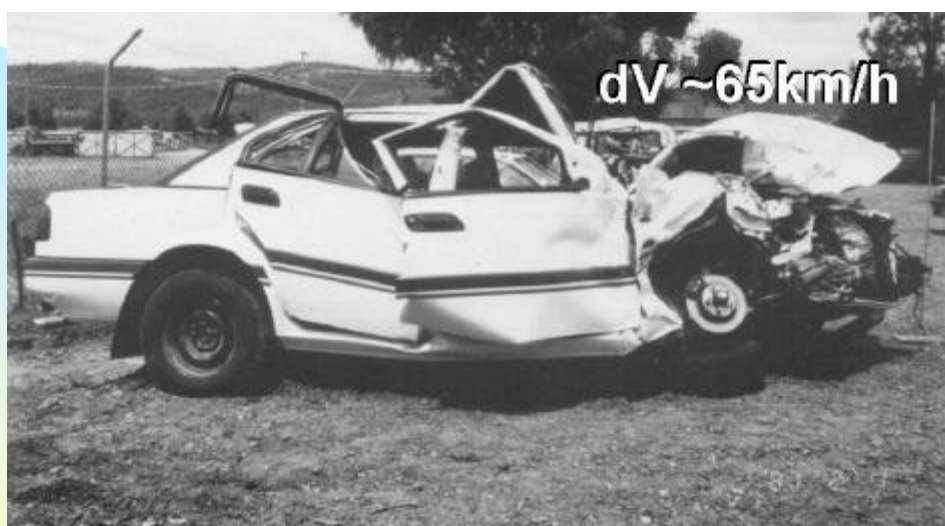
FIGURE 10 - 1992 Ford Falcon, change of velocity in frontal collision over 60 km/h; nine-month-old in forward-facing Type B seat sustained only bruising (27013)
