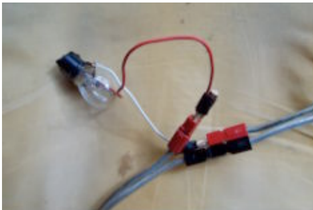
LEFT: Bulb seriesed between battery leads.
