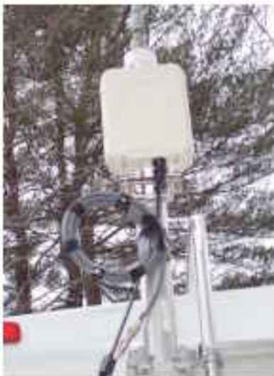
LEFT: Choke coil: Six in. dia. and 8 turns of coax at the tuner
