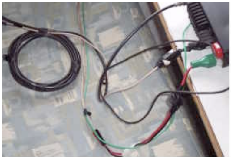
LEFT: Choke coil: Six in. dia. and 8 turns of coax at the tuner
