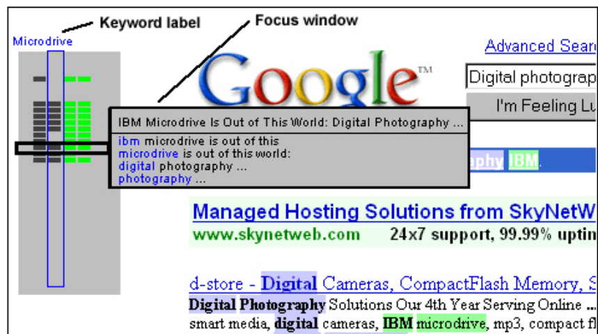
Figure 2 – The Vertical Context Lens: Rows represent segments and columns represent keywords. As the rows are smaller, brushing provides information for an entire segment. In this example, we are brushing a section containing 4 keywords. On top of the context window the CL shows the start of the segment for additional context. Note the keyword labeling in the CL. Also note that the CL is shown side by side with the base document in this case. The focus window floats on top of the Web page, which allows us to keep the CL very small.
