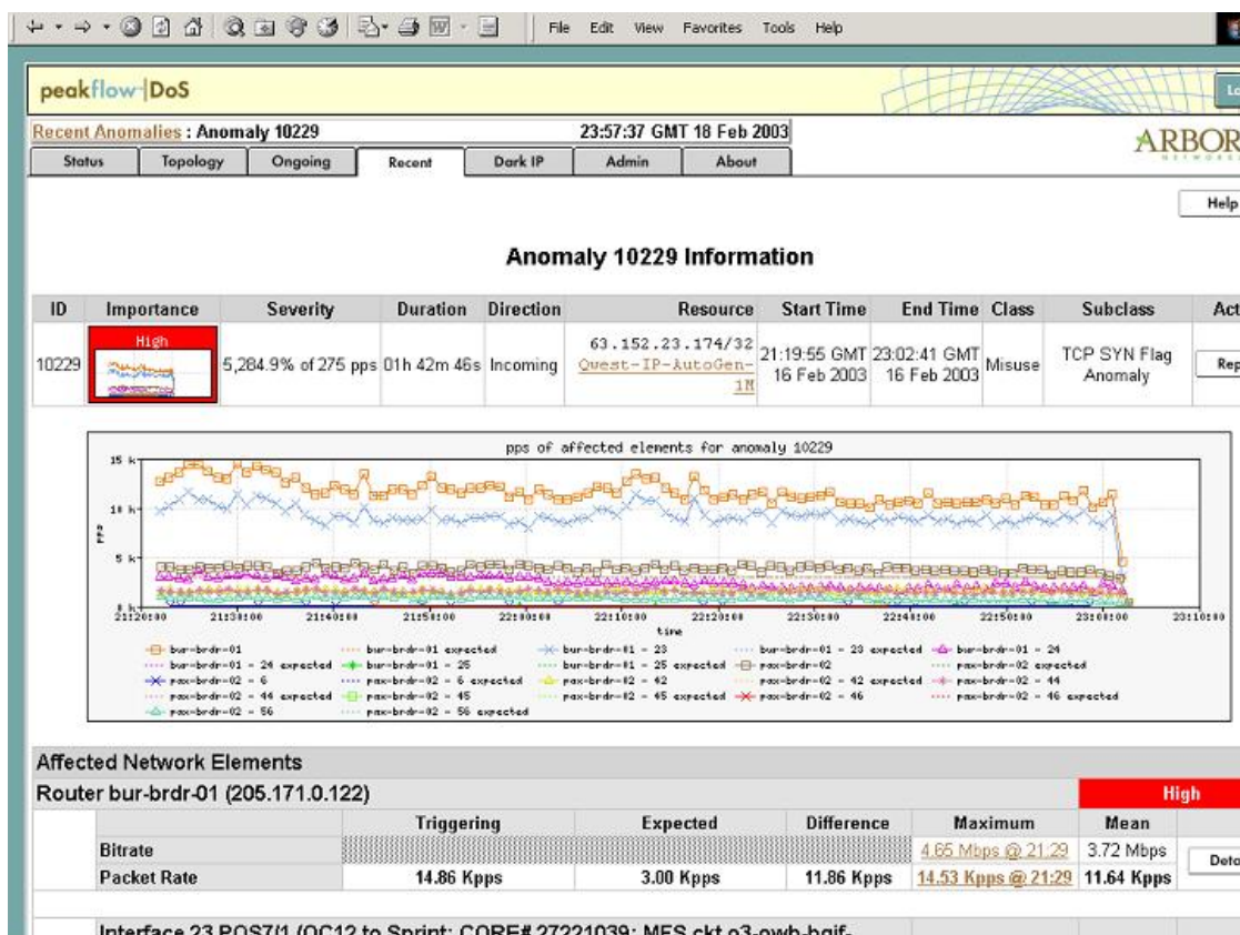
Figure 5 Sample Peakflow DoS Report for Anomaly Detection
