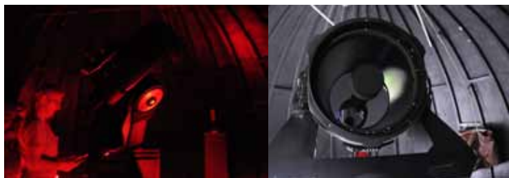
Chris Highlen, Phil Hudson and Dave Wilkins do fine tuning to increase scope stability, adjust setting circles and improve polar alignment.
